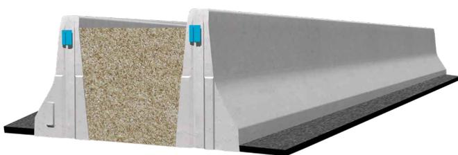
The double-row system is preferably used on the central reservation on motorways. The area between the elements is backfilled and the elements are additionally embedded 5 cm in asphalt, which guarantees a high protection against breakthrough. Despite the double-row and backfilled construction a working width of W5 is achieved.
